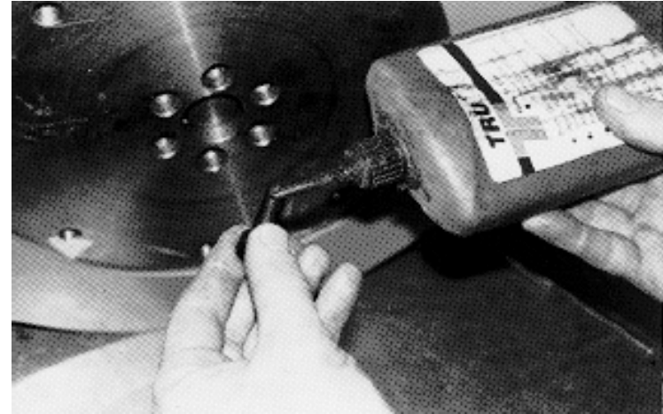
6. Remove old Lock-Tite compound from the socket head cap screws. Use one drop of stud grade Lock-Tite upon installation.
